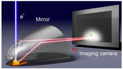
**Figure 1** Graphical representation of the angle-resolved CL imaging mode (image by Tremani).
